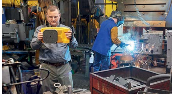
Fluke's ii900 Sonic Industrial Imager (acoustic imager) can pinpoint leaks from 50 metres away in a noisy environment.
