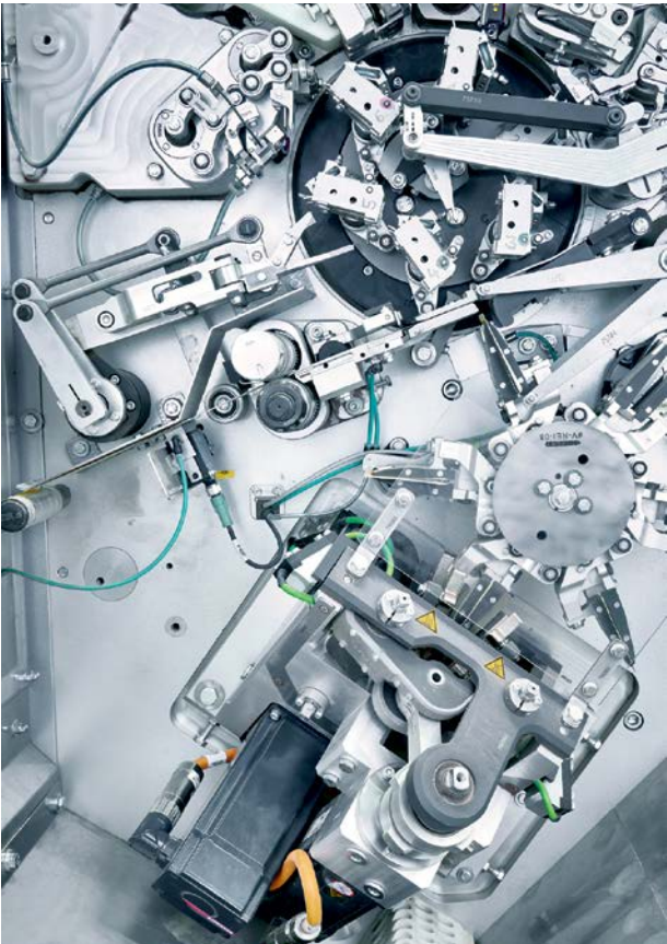
Control of the sophisticated kinematics via TwinCAT NC I and AM8000 servomotors increases the machine cycle as well as flexibility for bag geometry and different packaging materials.
