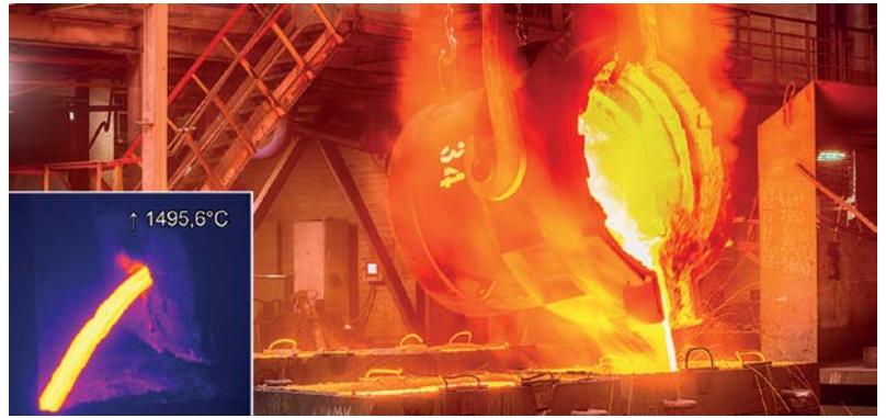
Optris IR cameras are designed to monitor temperatures in the metal casting process continuously.
