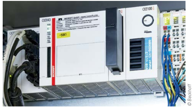
Dynamic synchronisation of all axes, safety, HMI, and individual database application – the complete automation project runs on a single CX2043 Embedded PC.
