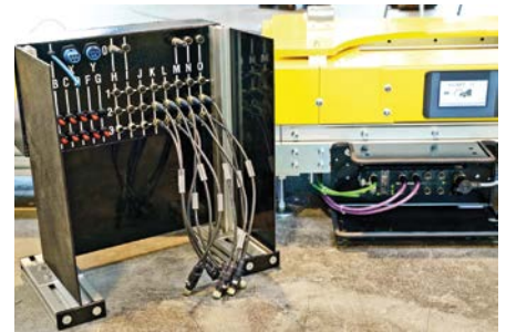
Before and after: The controller built in-house by Krups (left) worked well but, compared to Turck’s TBEN-L module (right), was much larger, more complicated to install and only worked in Profinet networks.
