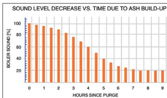
Figure 1 shows the rate at which sound level deteriorates over time due to fly ash build-up. The pipe sets need to be cleared at regular intervals to maintain effective leak detection.
