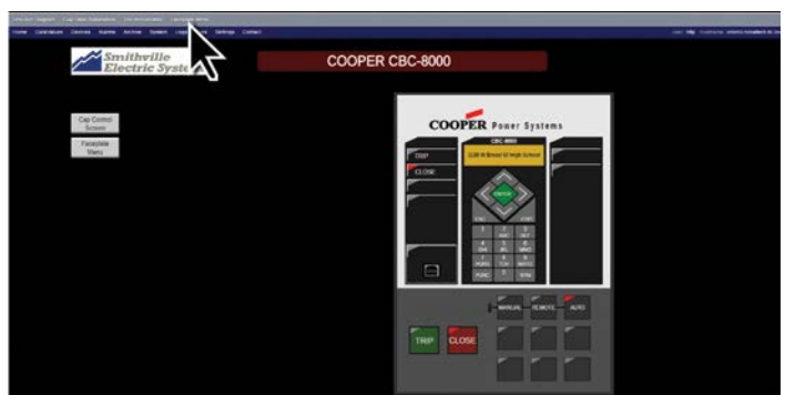
Operators can zoom into animated emulations of individual capacitor bank controllers and force controls.
