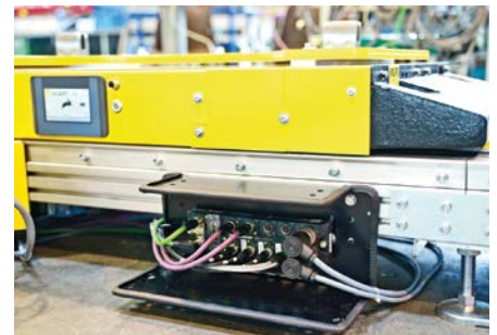
Turck’s TBEN-L-PLC controls the Krups conveyor system modules: communication to the periphery is via CAN and to the main controller via Profinet or Ethernet/IP.
