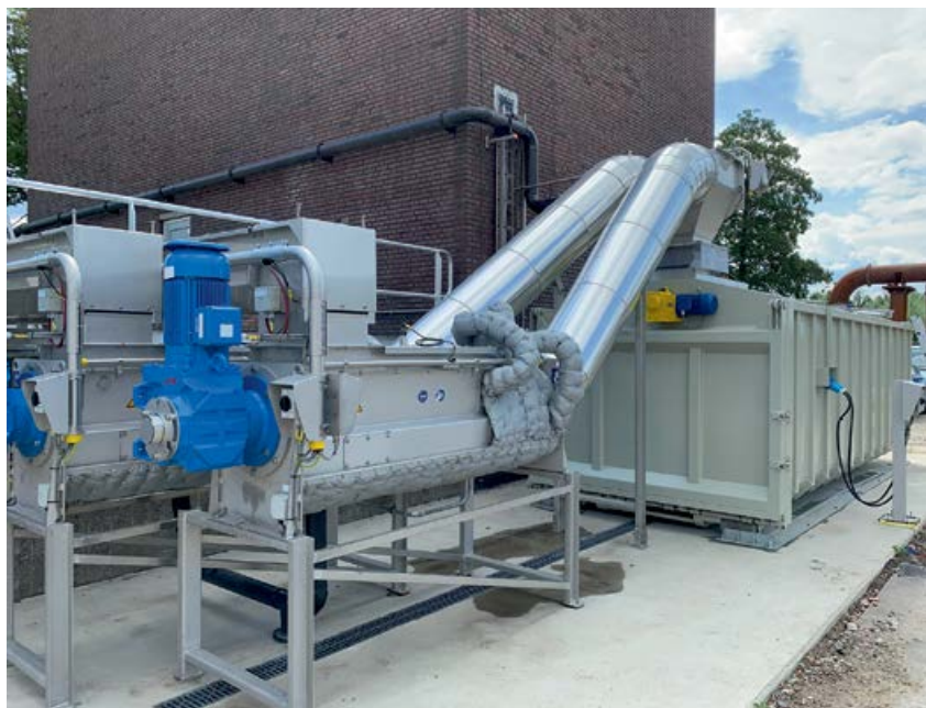
The new series of compact radar level sensors measures the level in the containers, without contact.
