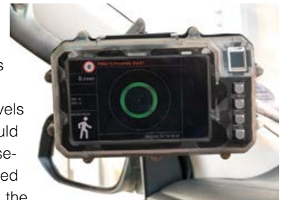
Collision Avoidance Systems used in surface mining have been developed to embrace technologies like satellite positioning systems, radar and smart vision.
