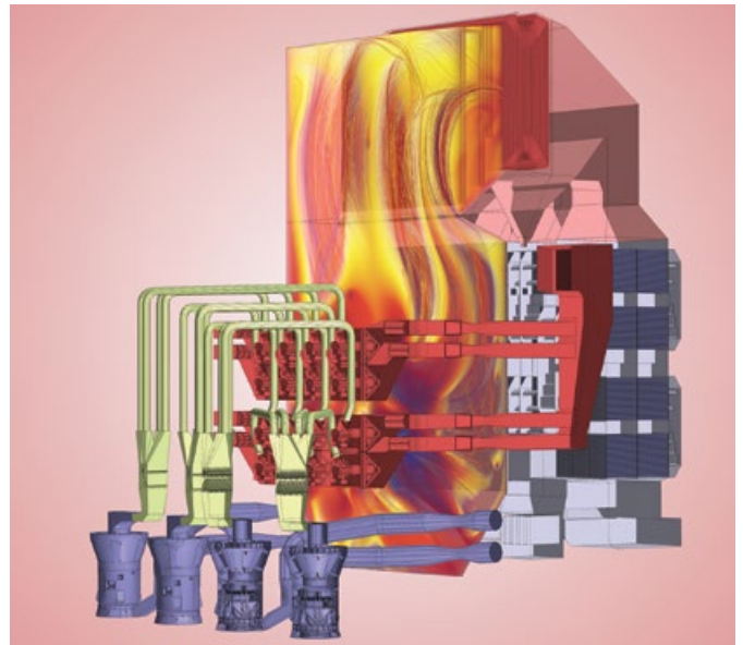
A CFD model of a boiler system including coal mills and pulverised fuel piping (foreground), burners and air ducting, furnace showing combustion flow paths and temperatures and downstream air heat exchangers (background).
