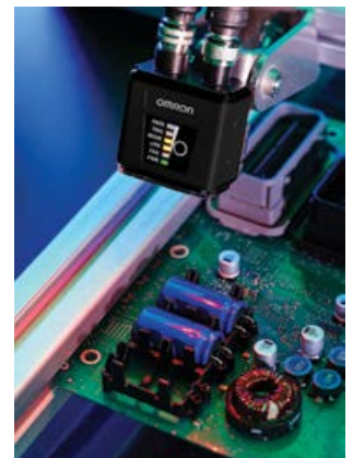
The compact V440 F can read dozens of tiny barcodes simultaneously.
