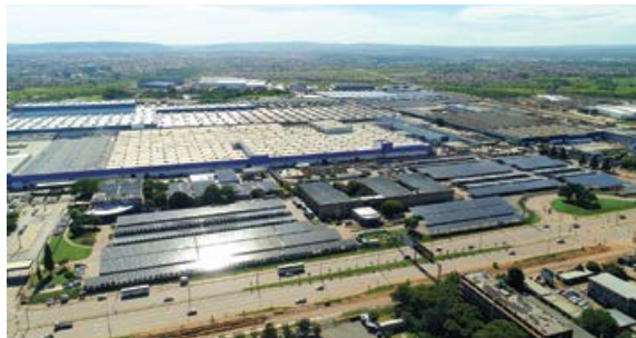
The 13.5 MW solar photovoltaic carport installation at the Ford assembly plant in Silverton.
