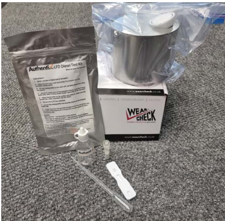
WearCheck's diesel test kit. Testing for illuminating paraffin in diesel is just one of many assessments offered by the company.
