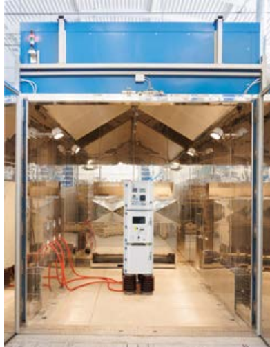
Testing unigear switchgear in the new climatic test chamber.
