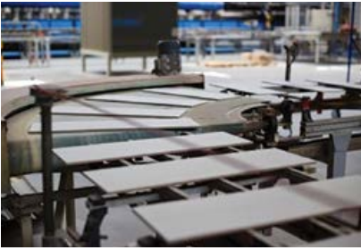
The tiles are transported through the manufacturing process by conveyor belt, automated via multi-axis motion controllers.
