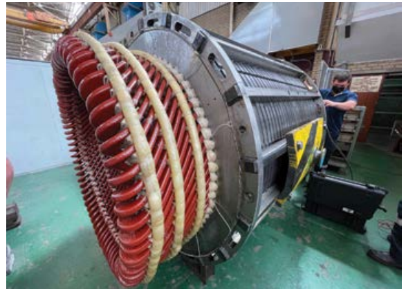
The 17 MW stator in preparation for testing.
