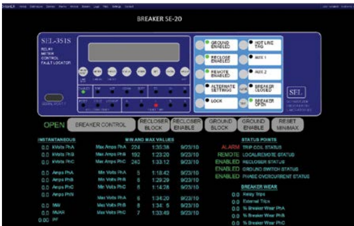
One-line diagrams in the Orion HMI show the status of the substation at a glance; feeder breaker zoom screens allow more detailed information to be viewed at the office.
