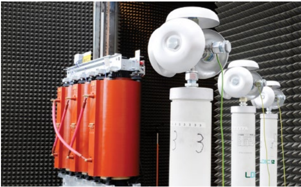
A cast resin transformer ready for acoustic level and partial discharge tests.
