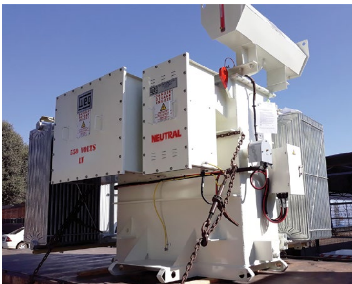
The locally manufactured 7 MVA transformer ready for transportation to site.
