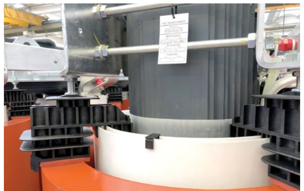
Fully assembled cast resin transformer, tag secured, with all fasteners torqued and marked.
