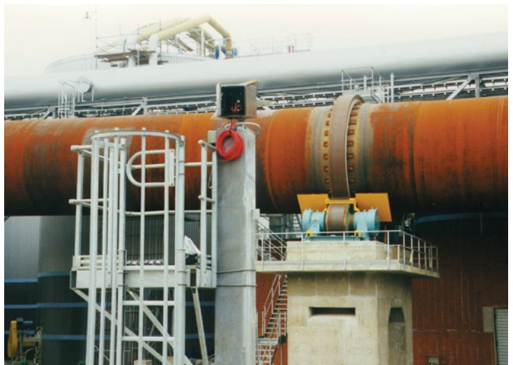
Ratio pyrometers which are designed for use in harsh environments support careful kiln management.
