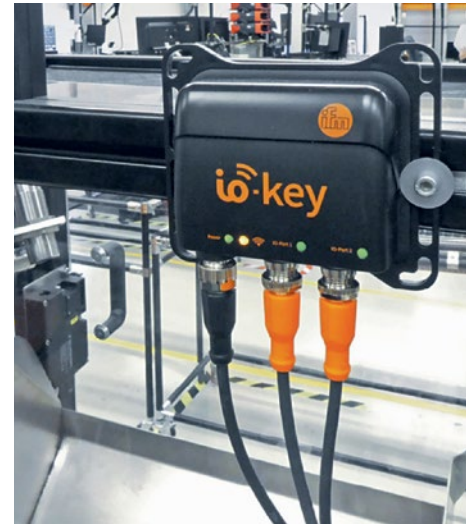
The IoT gateway is preconfigured, no sim card is required, to send sensor data via mobile network to the cloud.
