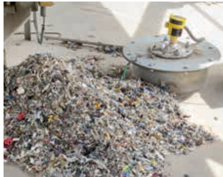
Despite the interference signals which could not be totally avoided, an almost exact level measurement is achieved with the VEGAPULS 69.
