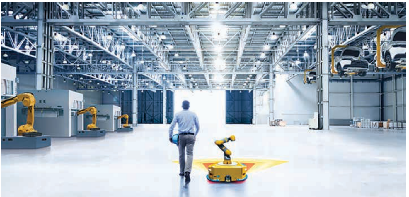
Mobile cobots mounted on automated guided vehicle systems are attracting interest in industry.
