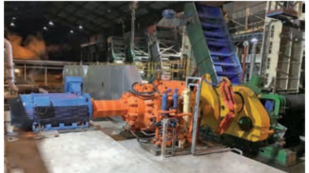
The TGM planetary gearbox and WEG motor at Green Fuel in Zimbabwe.
