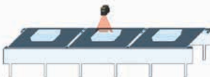
The laser-line triangulation sensor is used for rotation detection for ready-meal trays.
