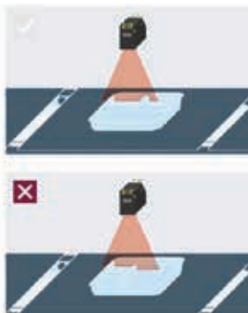
The laser-line triangulation sensor is used for rotation detection for ready-meal trays.
