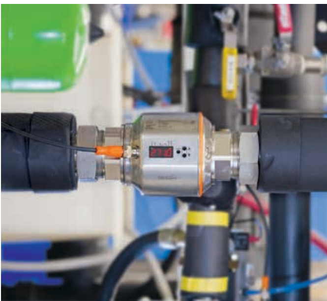
In water management applications, SM series flow meters measure water consumption.
