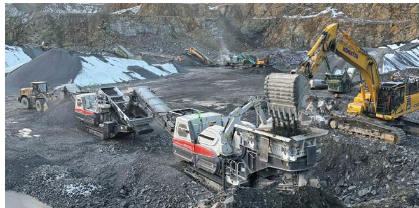
Left: Available in Southern Africa through Pilot Crushtec, the Metso Lokotrack LT400J combines high production capacity with improved energy efficiency. Right: The Metso Lokotrack LT400J introduces a new generation of high-capacity, diesel-electric primary crushing technology to Africa.
