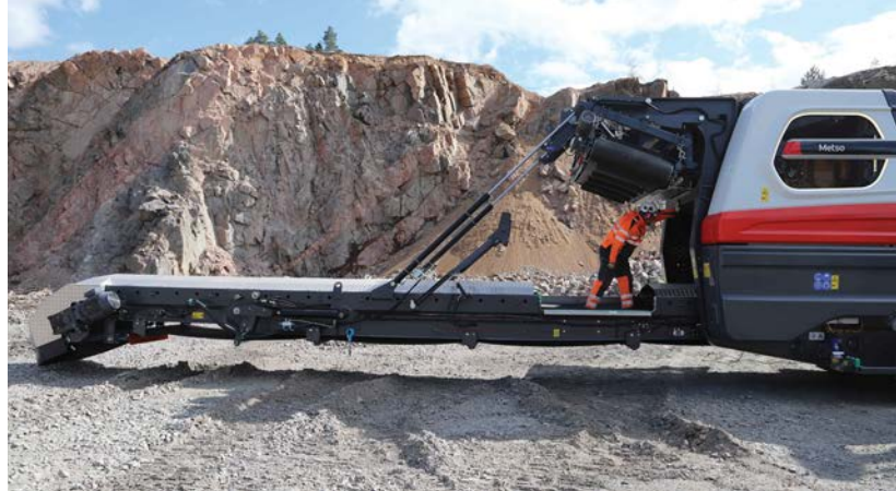
The extended discharge conveyor offers three operating positions, improving stockpiling flexibility and maintenance access.
