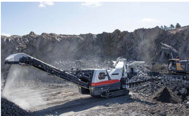
Left: Available in Southern Africa through Pilot Crushtec, the Metso Lokotrack LT400J combines high production capacity with improved energy efficiency. Right: The Metso Lokotrack LT400J introduces a new generation of high-capacity, diesel-electric primary crushing technology to Africa.
