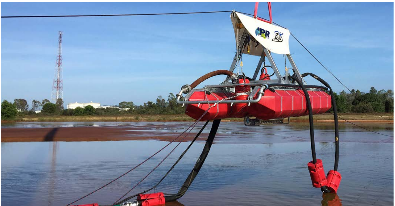
The SlurrySucker is mobile and can be deployed without interrupting ongoing operations.
