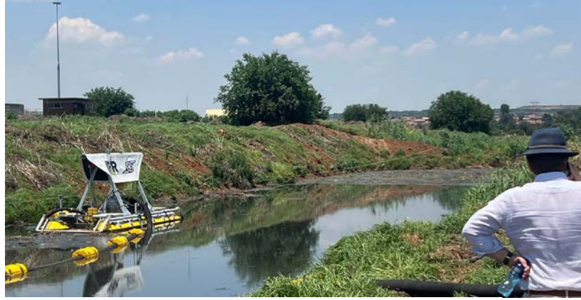
Left: The SlurrySucker removes silt quickly and without causing disruption to the dam's infrastructure. Right: The IPR SlurrySucker system is designed to remove sediment without damaging dam liners or disturbing the environment.
