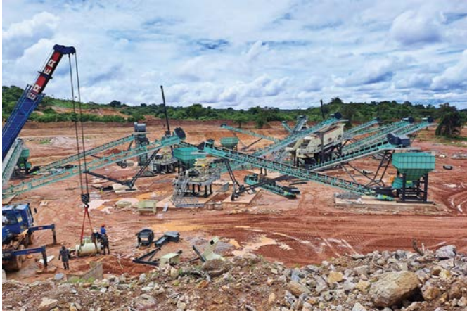
Left: The recently commissioned greenfields aggregate plant for Pilot Crushtec's customer in the Democratic Republic of Congo (DRC). Right: The Pilot Modular Nordberg HP300 cone crusher module.
