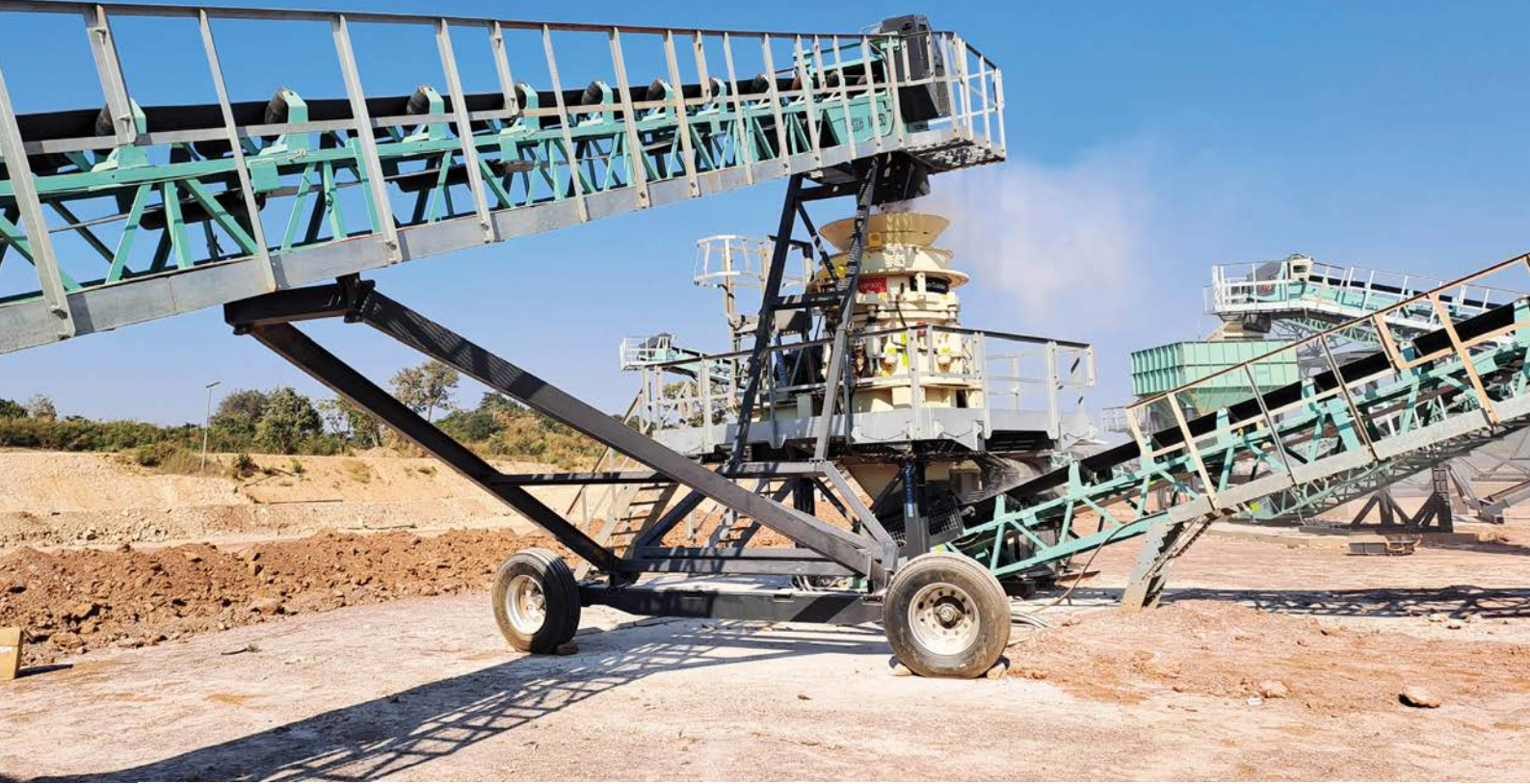
The Pilot Modular Feed Hopper MFH25 is used to control the feed to the cone crusher and an MPM910 magnet to remove tramp metal before the cone crusher.
