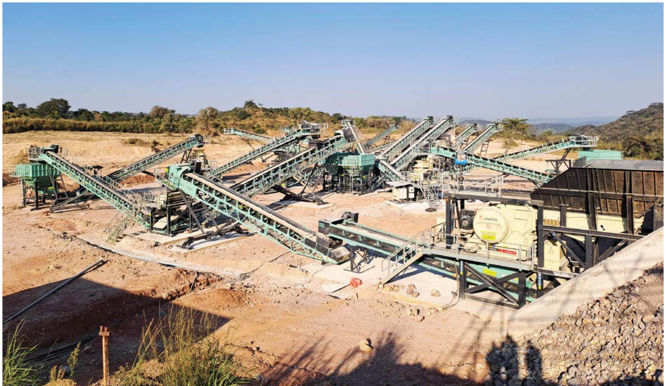
The 350 tonnes per hour (tph) production plant is the largest ever Pilot Modular aggregate production plant installation to date.
