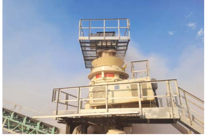
Left: The recently commissioned greenfields aggregate plant for Pilot Crushtec's customer in the Democratic Republic of Congo (DRC). Right: The Pilot Modular Nordberg HP300 cone crusher module.
