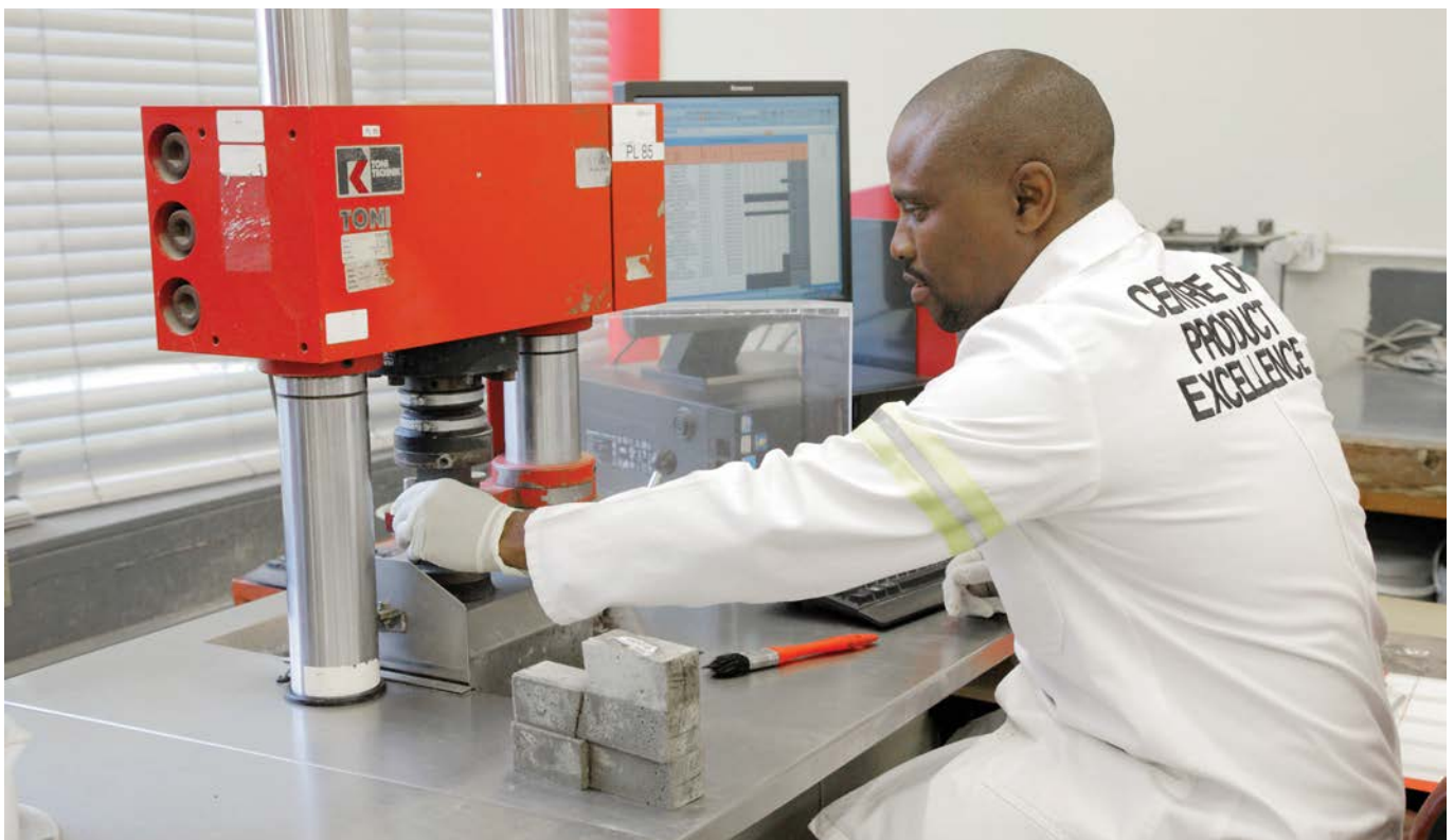
Customers like brickmakers can send their final products to the CPE for strength-class testing.
