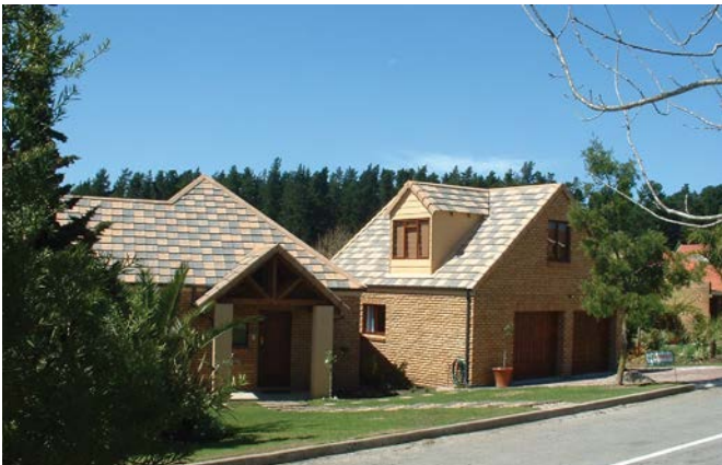
Left: One of the Western Cape’s most-loved concrete roof tiles, Eagle Roof Tile’s Shingle profile lends itself to the sharp triangular lines on this exposed intersecting gable roof. Right: Eagle Roof Tile’s slate grey shingle as seen on this A-frame with exposed gables in Eerste Rivier, Western Cape, was used to cover the roof and clad the vertical sides.
