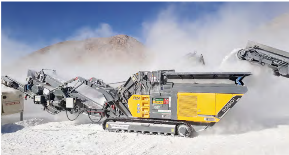
Rubble Master RM90GO! Is crushing marble aggregates on a quarry in Namibia.
