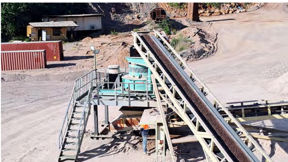
The recently commissioned Pilot Modular VS350 VSI module manufacturing sand in Botswana.
