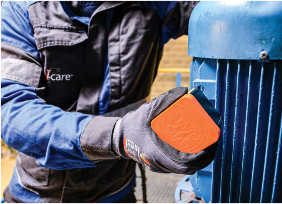
Online monitoring systems and remote sensors ensure that machinery is monitored without interruption.
