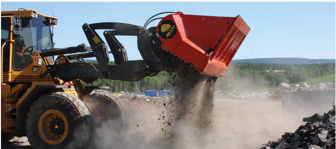
The ALLU recycling bucket sorts materials from actual waste and, in doing so, lowers transportation and landfill costs.
