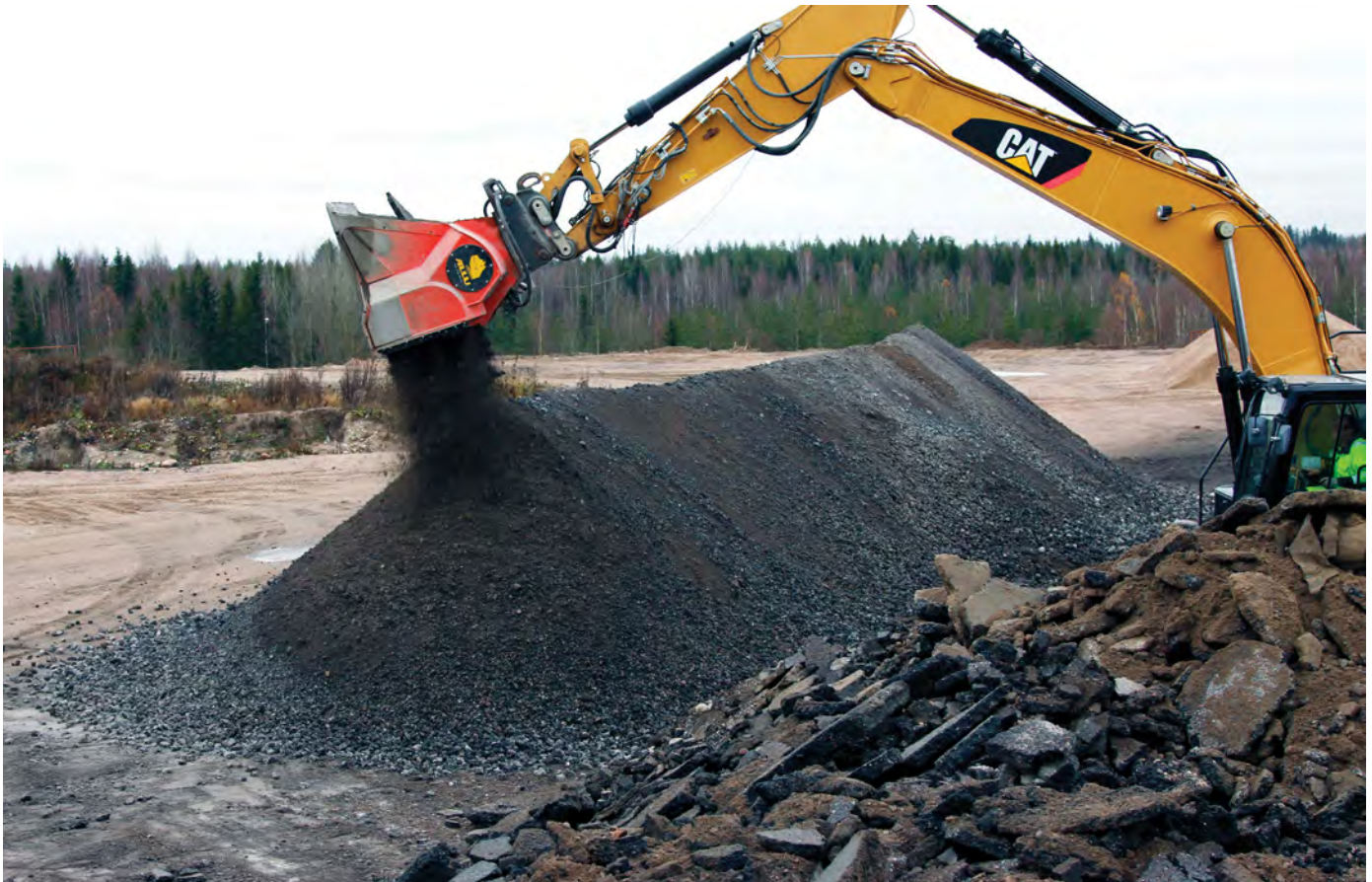
Bucket crusher attachments can turn carrier equipment into multi-purpose loading and crushing tools.
