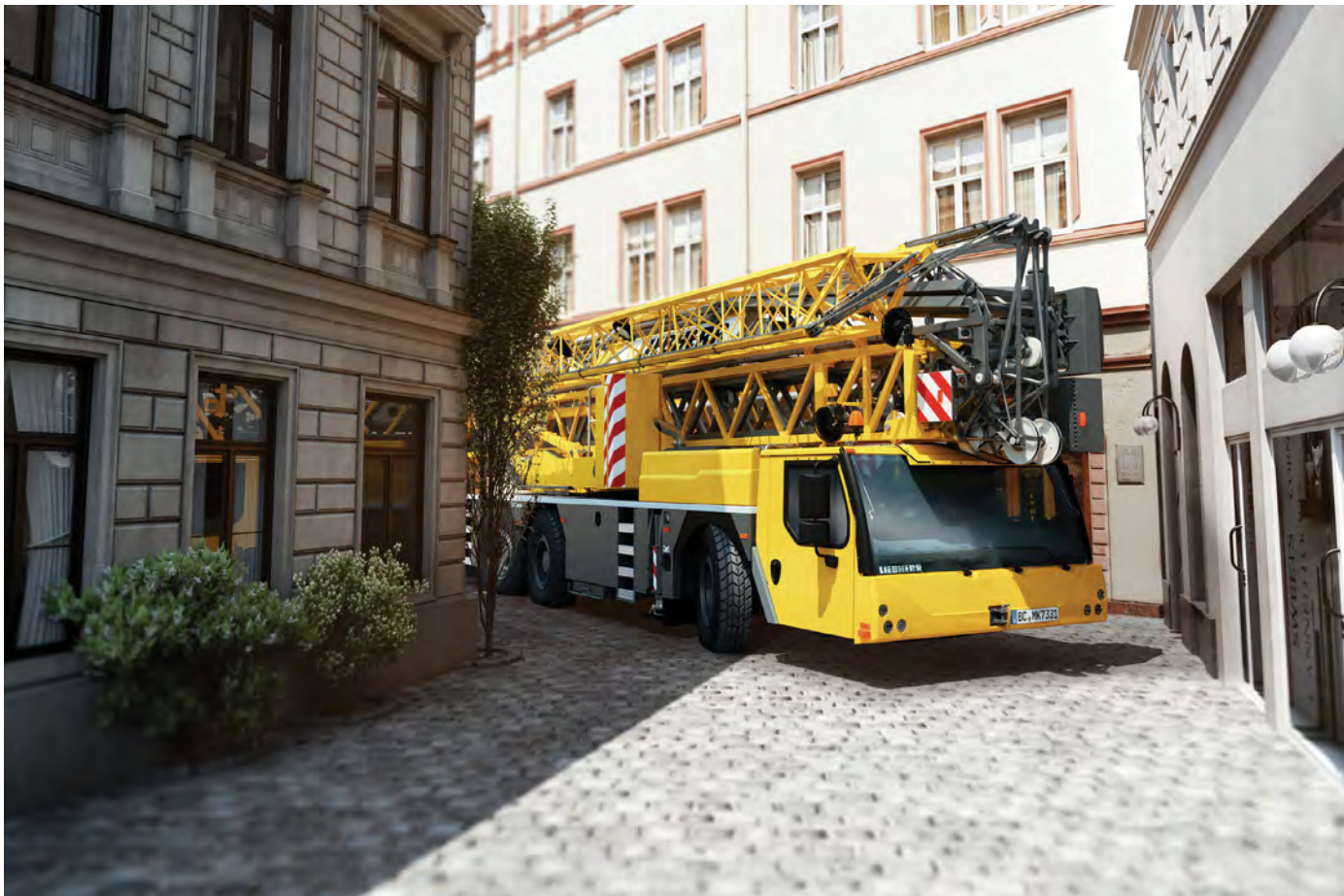
With a total length of 13,8 m, a width of 2,75 m and a height of 4 m, the Liebherr MK 73-3.1 is compact and easy to manoeuvre.
