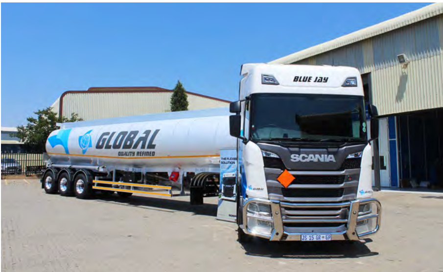
The new NTG R40 6x4 Highline has been supplied with an air suspension and Hazchem kit.
