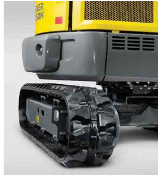
A key indicator of a poorly maintained undercarriage is the slapping noise in the case of rubber tracks due to low track tension.
