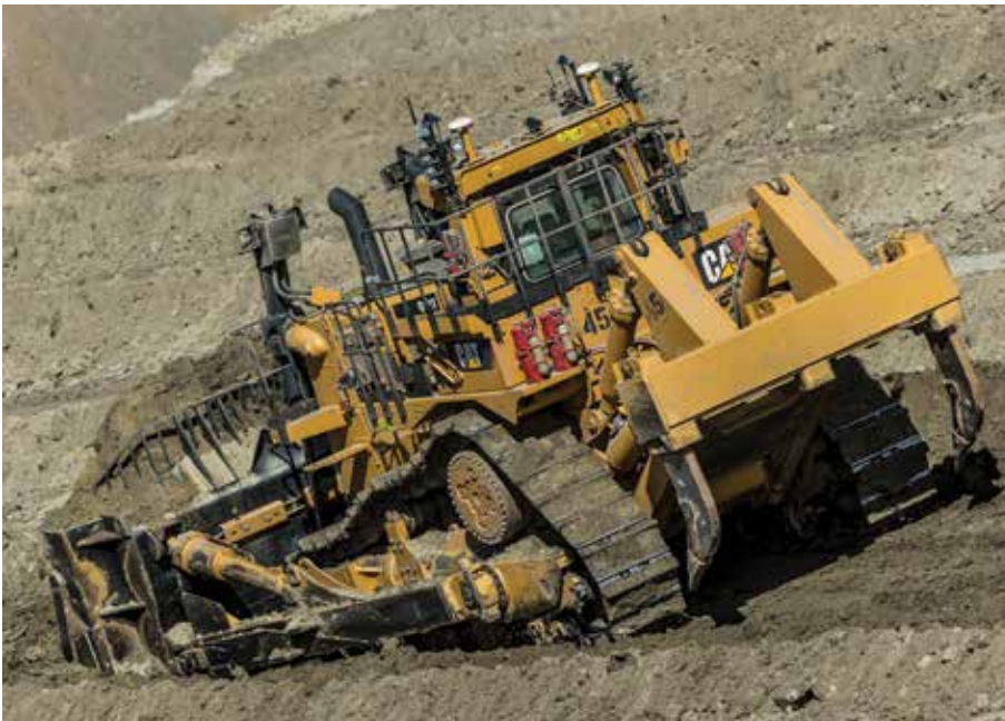
Command enables remote control and automation. Caterpillar now offers such systems for mining trucks, drills and dozers.
