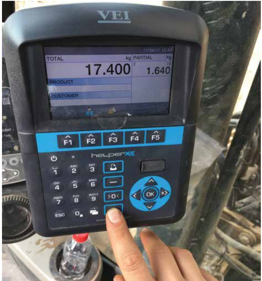
Various VEI models from DWS can be fitted on any machine with a lifting piston – from small forklifts to the largest rigid dumpers and excavators.
