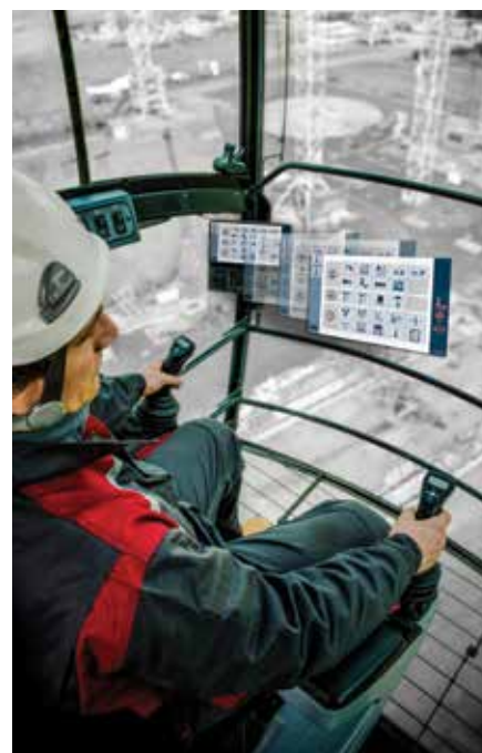
Potain Topless cranes are equipped with Manitowoc's Crane Control System, or CCS.
