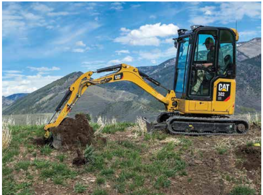
In an industry-first for 1-2 t mini excavators, models with a sealed and pressurised cab are available with air conditioning.
