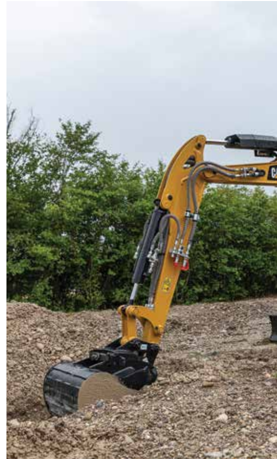
For added versatility, the standard auxiliary hydraulic system (complete with quick disconnect lines) provides one way, two-way and continuous flow.
