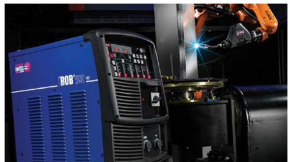
ABICOR BINZEL’s iROB modular robot power source series, tailor-made for the iBOTone cobot system, provides the full range of welding power.
