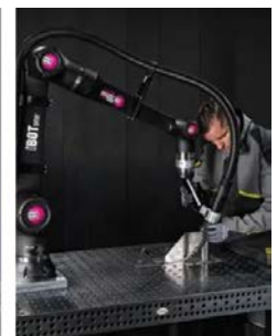
With its self-explanatory, intuitive operation, unmatched repeatability of within 0.02 mm across all applications, and exceptional flexibility, iBOTone® is an ideal solution for welding production environments that require small batches of different products.
