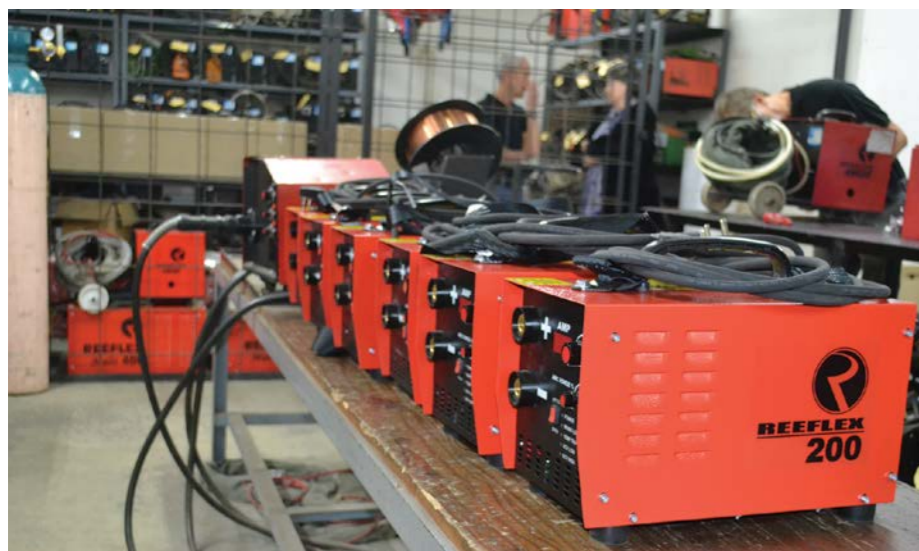
Single phase 200 A ARC Inverter Welders being manufactured at Reeflex's Randburg manufacturing facility
