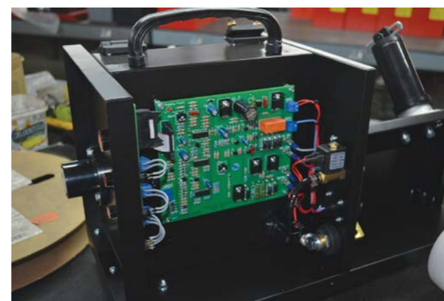
A key design decision was to continue to use through-hole PC boards for the electronics, which makes it easy for anyone to find a fault and repair it.
