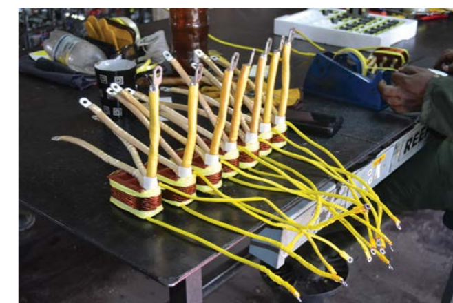
The transformers used for Reeflex welding inverters are manufactured onsite using a winding machines and techniques developed in-house.
