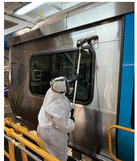
Nitty Gritty surface-cleaning and polishing machines with wide brushes are ideal for cleaning the sides of stainless-steel railway vehicles.
