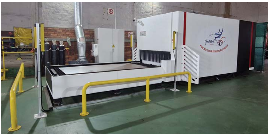
Jubilee Suppliers' new 6.0 kW Jinan Acme CNC cutting system, recently acquired from Cosmo Group, features a Max Photonics fibre-laser cutting head, a 3.0×1.5 m double-exchange worktable, and a fully enclosed laser-cutting area.
