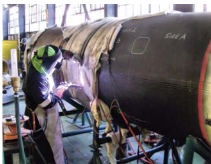
Above: For piping with wall thicknesses up to 6.0 mm, Aurex typically use GTAW, which allows for precise control and high-quality welds with minimal rework. Right: On thicker-bore piping with wall thicknesses exceeding 10 mm, Aurex consistently achieves rejection rates below 2.5%.
