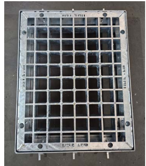
Jubilee Suppliers manufactures, under licence, a patented grid for storm water drainage. The bars are precision-cut with slots, assembled into a grid, and then welded at the end of each bar to secure the grid structure.
