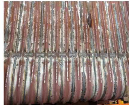
A boiler membrane wall panel. For long structural welds, SteinMüller uses a qualified metal-cored wire procedure. Laser cleaning is used before welding, and a weld prep primer is added after.
