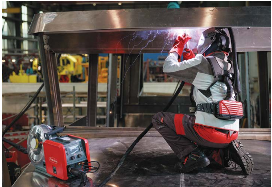
The split Fortis, equipped with an external wire feeder, ensures a maximum operating range of up to 20 m with an interconnecting hose pack. The Pulse function can also be used with an intermediate hose pack up to 15 m long.
