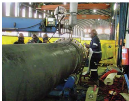
Above: For piping with wall thicknesses up to 6.0 mm, Aurex typically use GTAW, which allows for precise control and high-quality welds with minimal rework. Right: On thicker-bore piping with wall thicknesses exceeding 10 mm, Aurex consistently achieves rejection rates below 2.5%.
