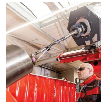
Above: Fronius' tilting positioner with an ETR (Endless Torch Rotation System) offers unlimited rotation and positioning of the welding head.
