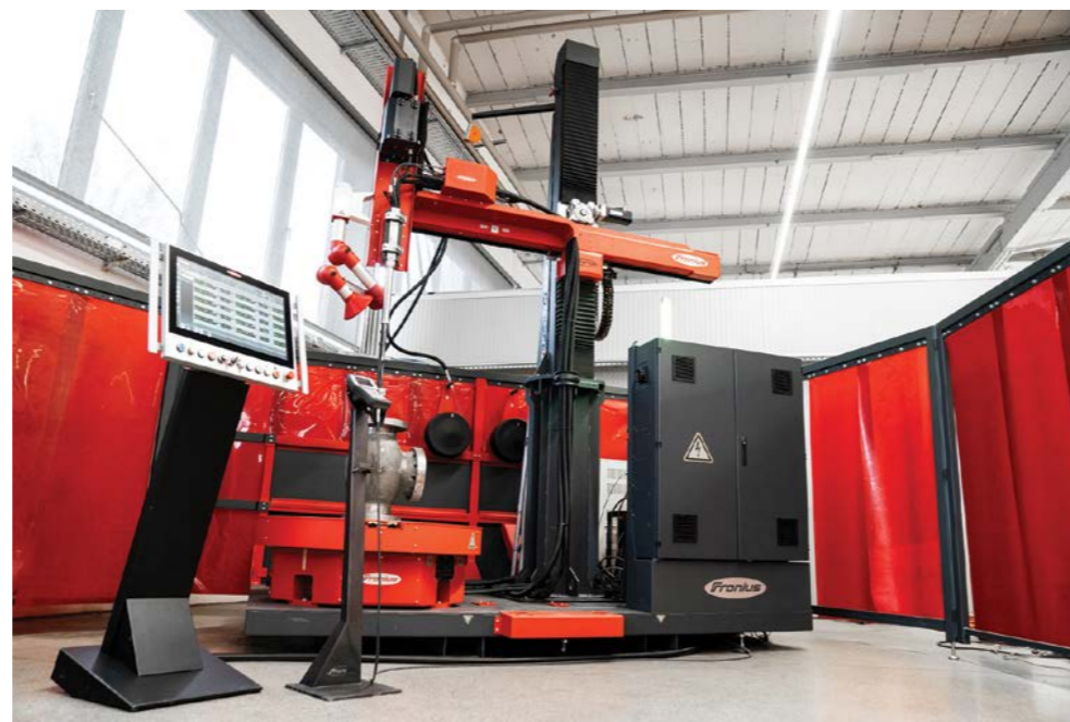
Above: Fronius' tilting positioner with an ETR (Endless Torch Rotation System) offers unlimited rotation and positioning of the welding head.
