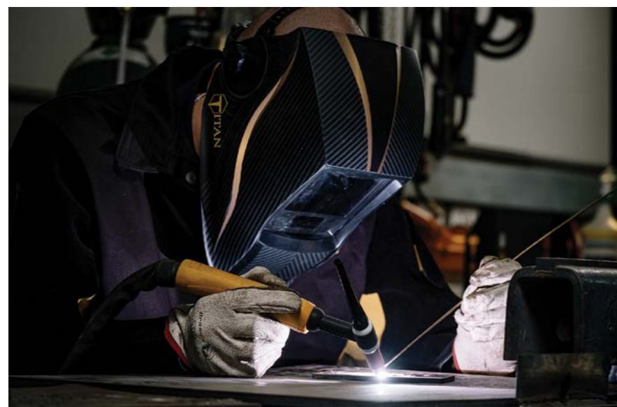
Thermamax TITAN helmets with auto-darkening filters (ADFs) are able to automatically adjust the sensitivity level to set the right level of protection. Left/Above: TIG welding; Left/Above: MIG/MAG welding.
