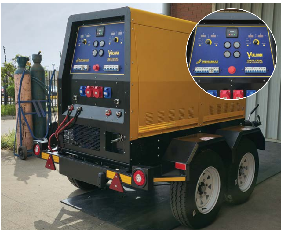
The core of the package includes two highly efficient 600 A multi-process welding inverters driven by a Perkins genset. Inset: The system has been made very easy to operate with only one process selection switch and one welding power setting per welding inverter on the front panel.
