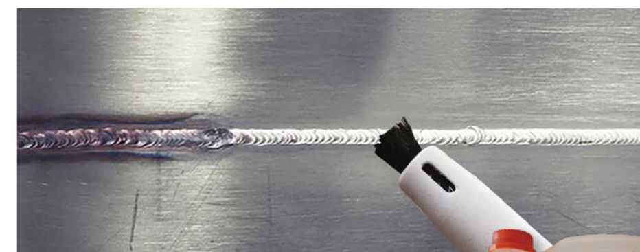
Above: This process will not only remove imperfections on the surface that the welding process has caused, but it will instantly restore the passivating oxide layer required to return the stainless steel back to its protected state.
