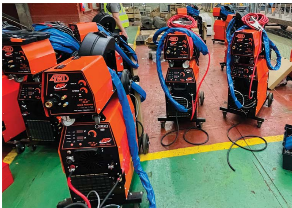
The Starweld CC/CV Quatro power sources delivered to Transnet. These machines are tunnel cooled to prevent contaminated cooling air passing over electrical and other components in the machine.
