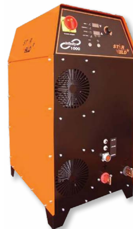
The Starweld 1 000 A INFINITY submerged arc welder developed for the yellow metal industry.
