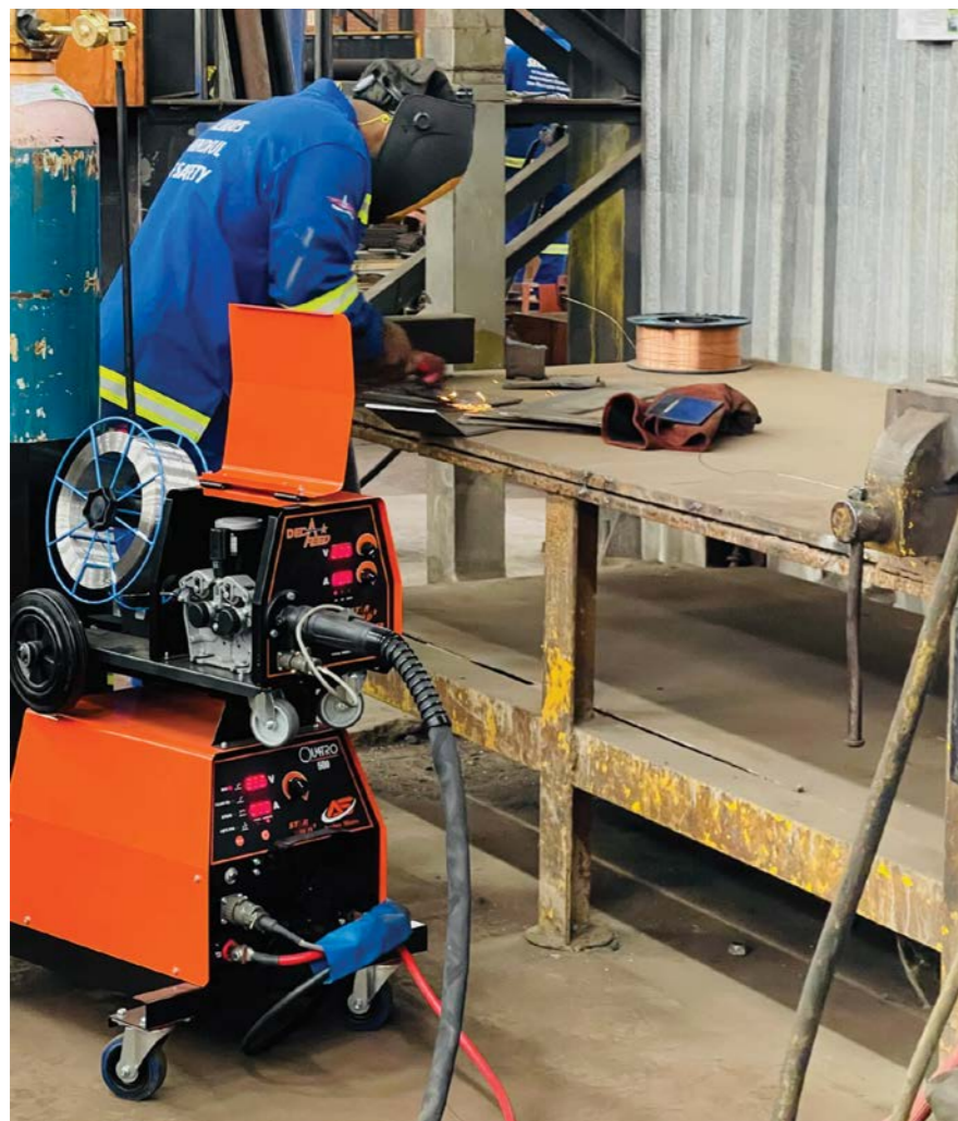
The Starweld digitally controlled Deca Feeder Series, was also introduced for use where precise welding parameters needed to be recorded.
