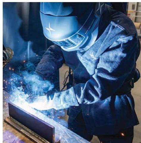
In trials comparing the new diamondspark GUARD 420 MC metal-cored welding wire with the standard diamondspark MC wire, operator exposure to airborne Mn was significantly reduced, helping fabricators to meet recently revised exposure limits.
