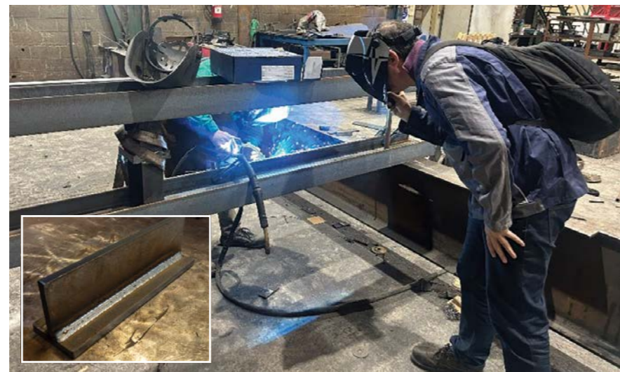
The seamless diamondspark GUARD 420 MC wire on trial at a shipyard. Inset: diamondspark GUARD wires provide the same level of welding productivity and welding performance as conventional diamondspark cored wires, with a substantial reduction in the manganese content in the welding fumes.
