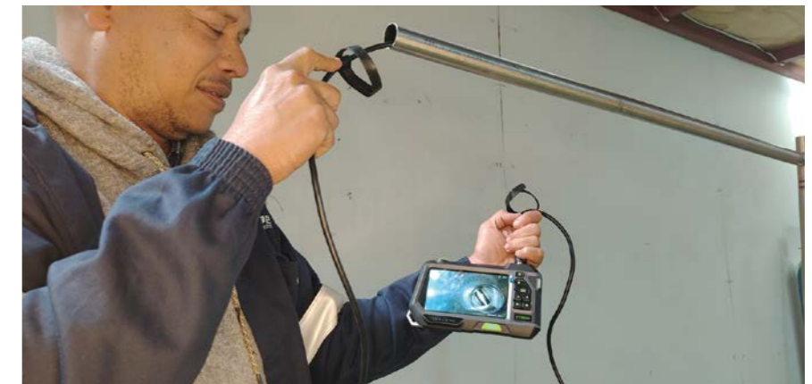
Borescope inspection is regularly used to determine the finished quality of the inside surfaces of tubes and pipes.
