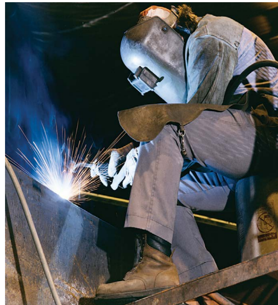
It is important to match a shielding gas mixture to a GMAW or GTAW application to achieve the best results possible, says Sean Young.
