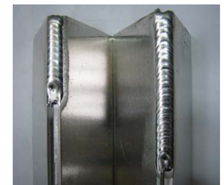
A 20 second aluminium TIG/GTAW welding comparison on thicker section plate using accurate current at 150 A. Left: 100% Ar; Right, Ar+He.
