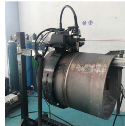
In combination with diamondspark flux cored wires, pipeRunner® can produce excellent girth welds of the highest quality, minimising NDT indications and lowering repair rates.
