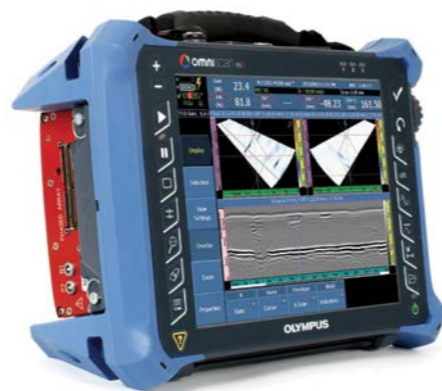
Phased array UT uses a probe with 64 or 128 separate transducer elements to enable every probe angle to be covered at the same time, which enables the whole weld profile to be tested at the same time.
