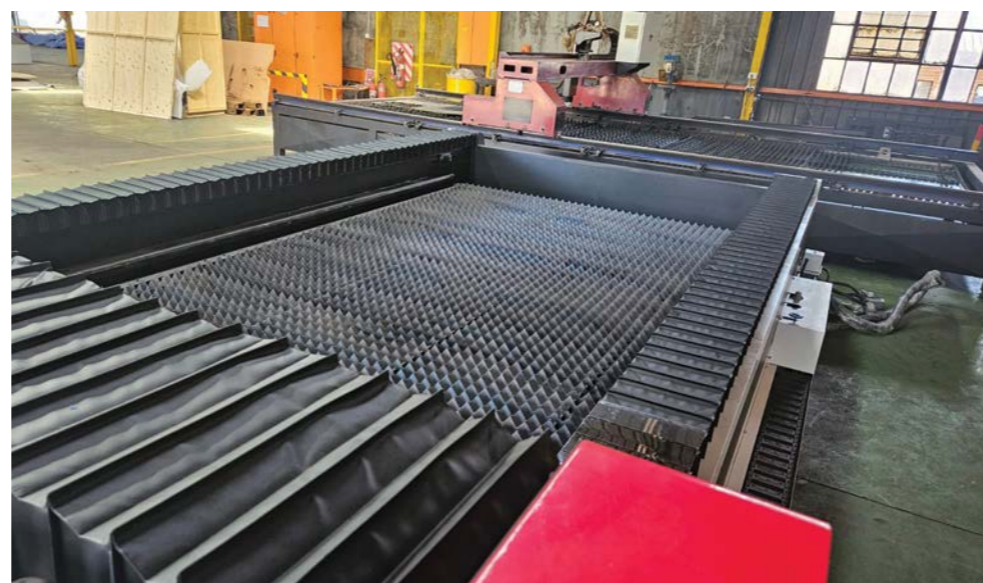
The bed is a heavy-duty, double-exchange, automatic feeding table that is precision milled. While cutting one sheet, the next sheet can be loaded ready to be moved into place.
