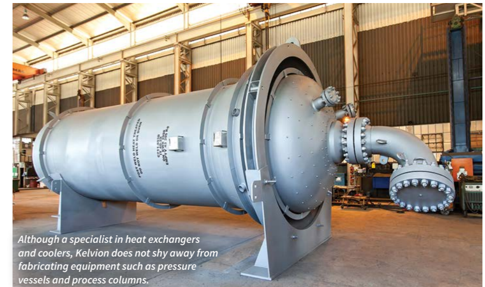
A 316L Stainless Steel Channel for a heat exchanger.
