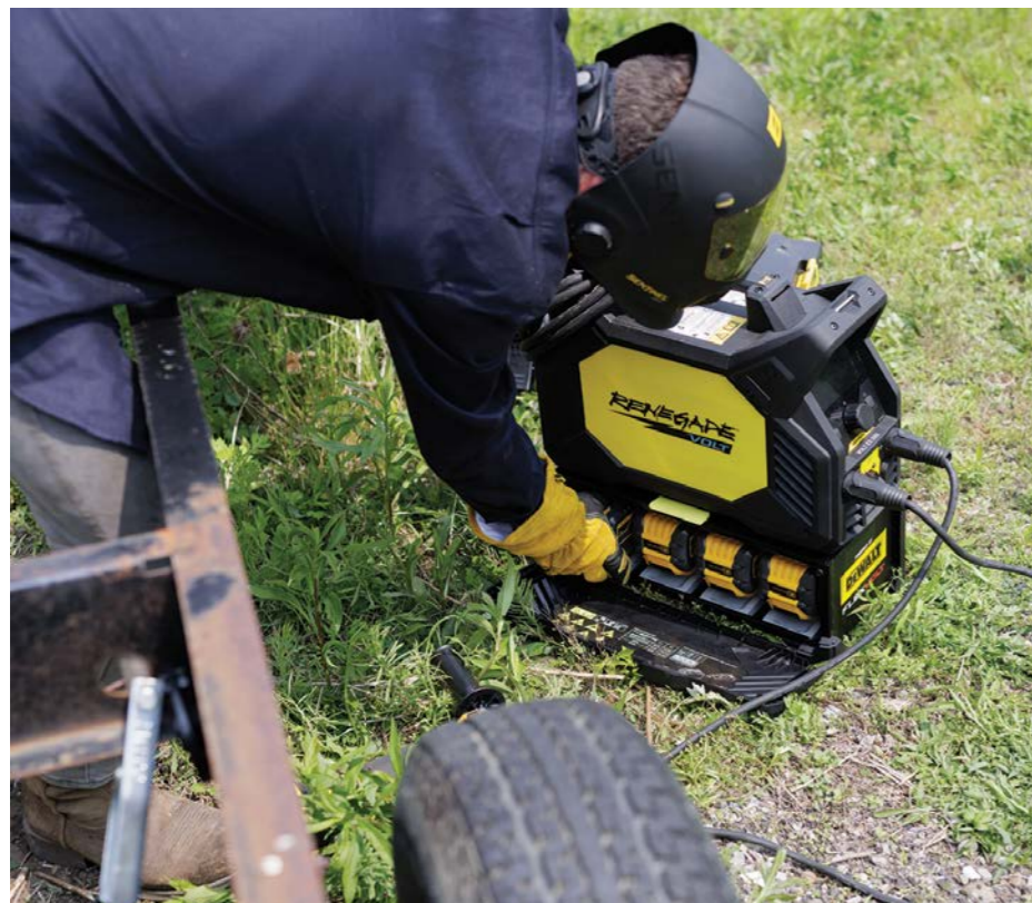
ESAB’s new Renegade VOLT™ ES is a portable, cordless battery powered, Stick (SMAW) and Lift TIG (GTAW) welder that uses four 12 Ah DeWalt batteries to provide enough the power to consume up to 33 E6013 electrodes on a single charge.
