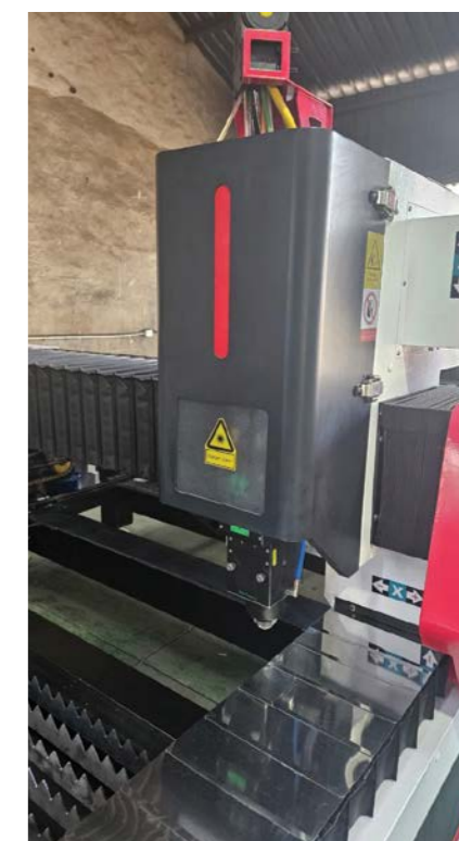
The laser source is a Max 6.0 kW fibre laser, a premium Chinese brand, while the laser head is a 6.0 kW Raytools BM06 K.
