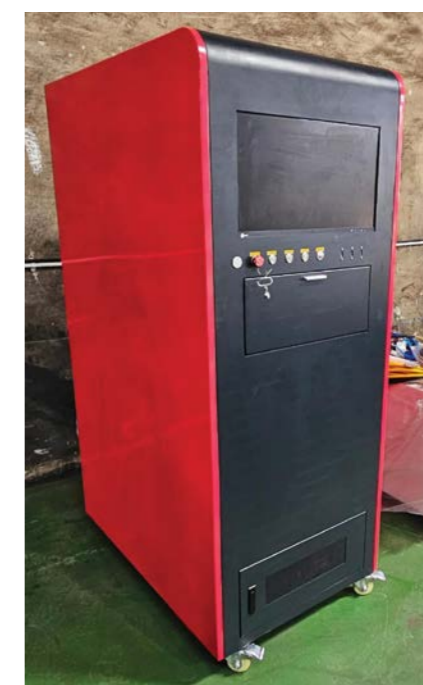
A FScut 4000E control system that incorporates the CNC, cutting and nesting software ensures easy operation with fast, accurate and clean cut quality.
