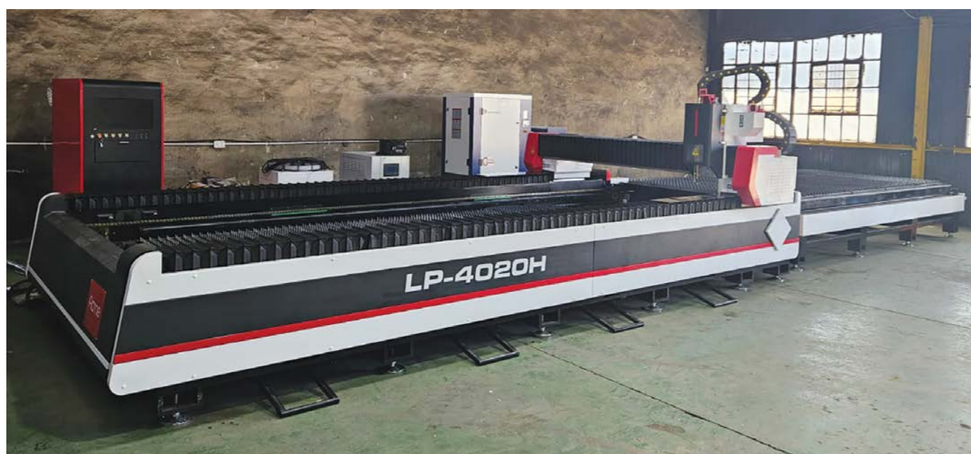
MD Steel is now using the machine to cut material using a 20 mm nozzle that can handle a 20 to 26 mm cut.
