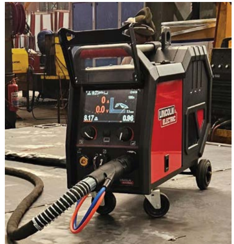
The advanced Lincoln Electric LF56D wire feeder, with its high-efficiency COOLARC® 60 water cooler, was chosen to ensure continuous welding.
