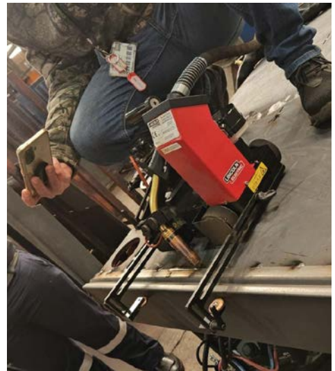
For WELDYCAR, Lincoln Electric has developed a set of magnetic and other guiding systems that eliminate the need to continuously adjust the carriage position while welding.
