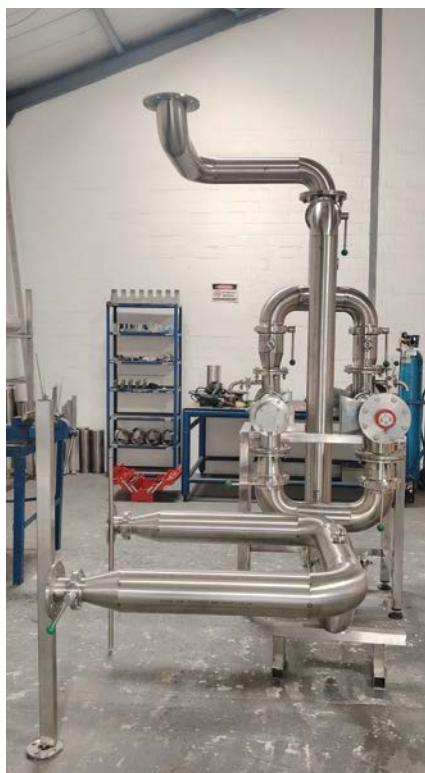
A UHP fabrication for Coca-Cola being completed at Sanipipe's Cape Town facility.
