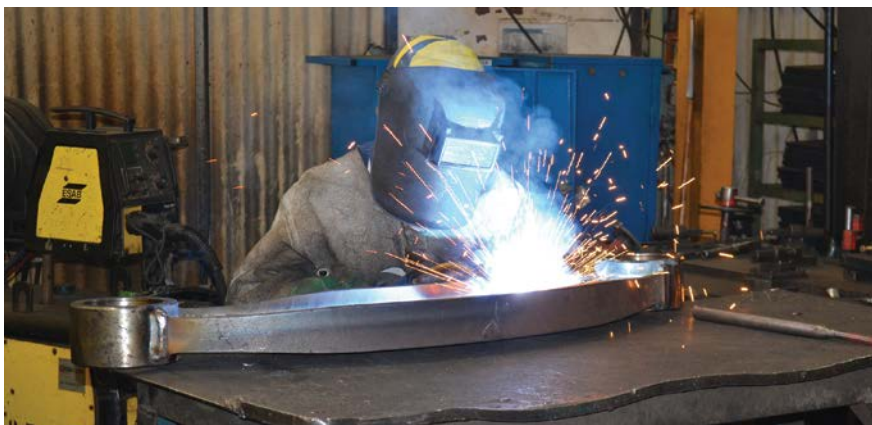
Most of the welding at BHI is done using the down hand (1G, 1F and 2F) positions, where solid wire, gas metal arc welding (GMAW) is preferred.
