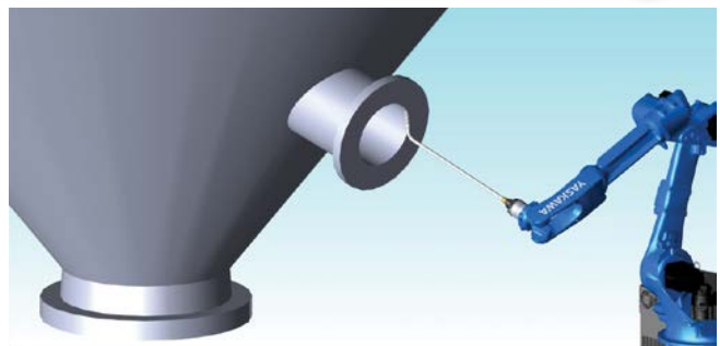
A 3D CAD model of Yaskawa Southern Africa’s nozzle cladding system being developed for Hydra-Arc.
