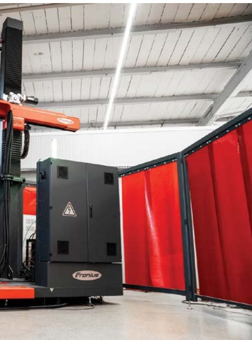
Above: Fronius' tilting positioner with an ETR (Endless Torch Rotation System) offers unlimited rotation and positioning of the welding head.
