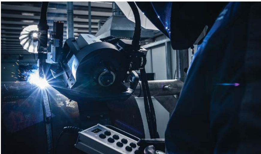
In combination with diamondspark flux cored wires, Böhler Welding's pipeRunner® for pipeline welding can deliver flawless girth welds with excellent material properties.
