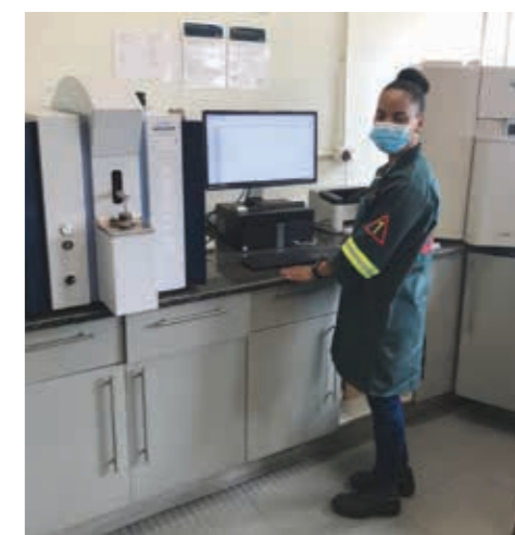
Laboratory Supervisor, Lydia Motaung, at the spectrometer for testing weld-metal chemical compositions of test specimens.
