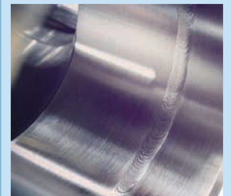
An example of the bright surface finish on the inside of a pipe protected using HFT's Weld Purge Plugs.
