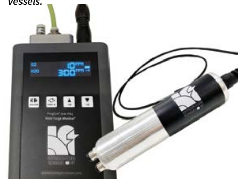
Figure 6: A weld purge monitor showing O 2 and H 2 O levels.
