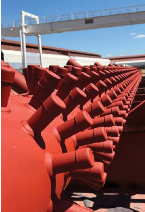
Steinmüller Africa’s header nipple welder with two submerge arc heads and an inner fusion TIG head, with each head able to travel across a 28 m length. Right: A completed header manufactured by Steinmüller Africa in Pretoria North as part of its Medupi and Kusile new-build contract.
