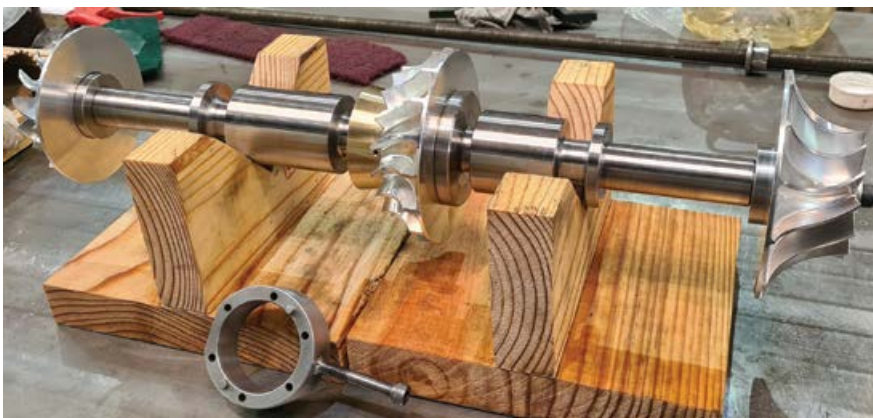
A new and complete turbine rotor reversed engineered and manufactured based on the data extracted from a damaged component.
