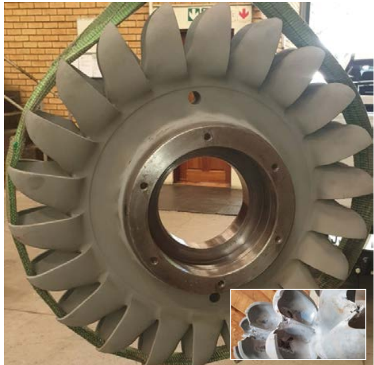
A fully refurbished Pelton wheel for a water-turbine re-engineered and refurbished in 316 stainless steel from the damaged original (inset).
