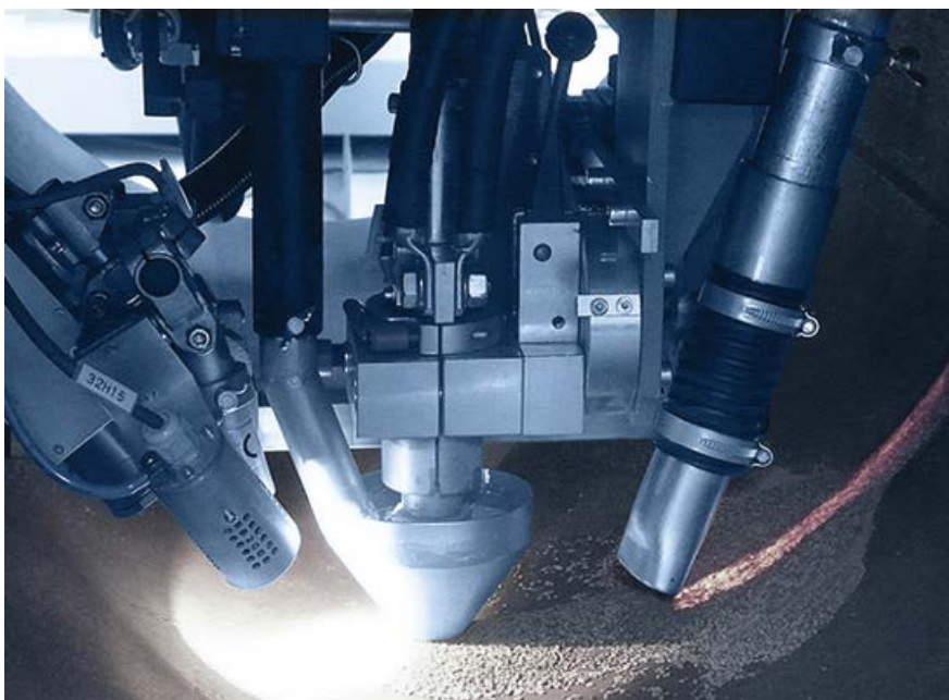
voestalpine BÖHLER Welding's SAW range of cored wire and flux combinations offer the welding performance and quality required for the manufacture of offshore and onshore wind towers.
