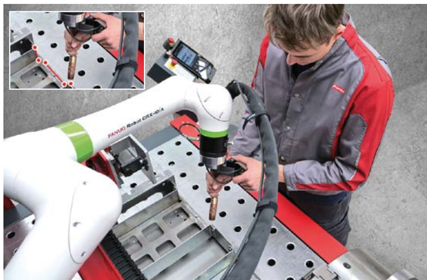
No programming knowledge is required for teaching the cell – the programming steps are intuitive and easy to learn, allowing the welding specialist to concentrate on more challenging tasks. Inset: The welding path is established point to point on the component. The software then uses these key points to calculate the welding contours and welding sequence. Photos courtesy of Fronius International.
