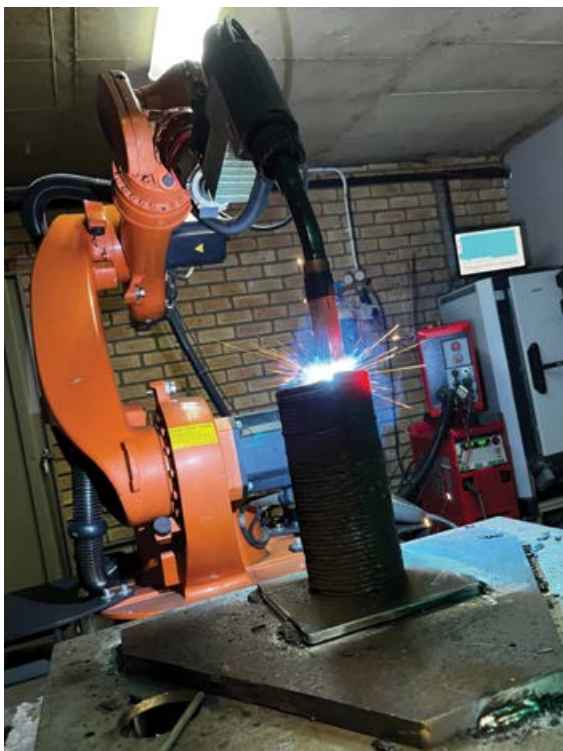
A KUKA robot arm is used with Fronius’ Cold Metal Transfer (CMT) welding process for 3D printing/additive remanufacturing of high-value replacement components and rapid prototyping of products in the development phase.
