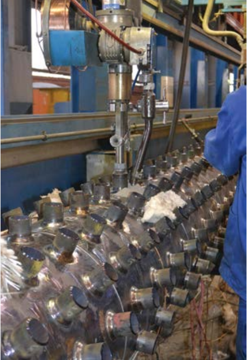
Steinmüller Africa’s header nipple welder with two submerge arc heads and an inner fusion TIG head, with each head able to travel across a 28 m length. Right: A completed header manufactured by Steinmüller Africa in Pretoria North as part of its Medupi and Kusile new-build contract.
