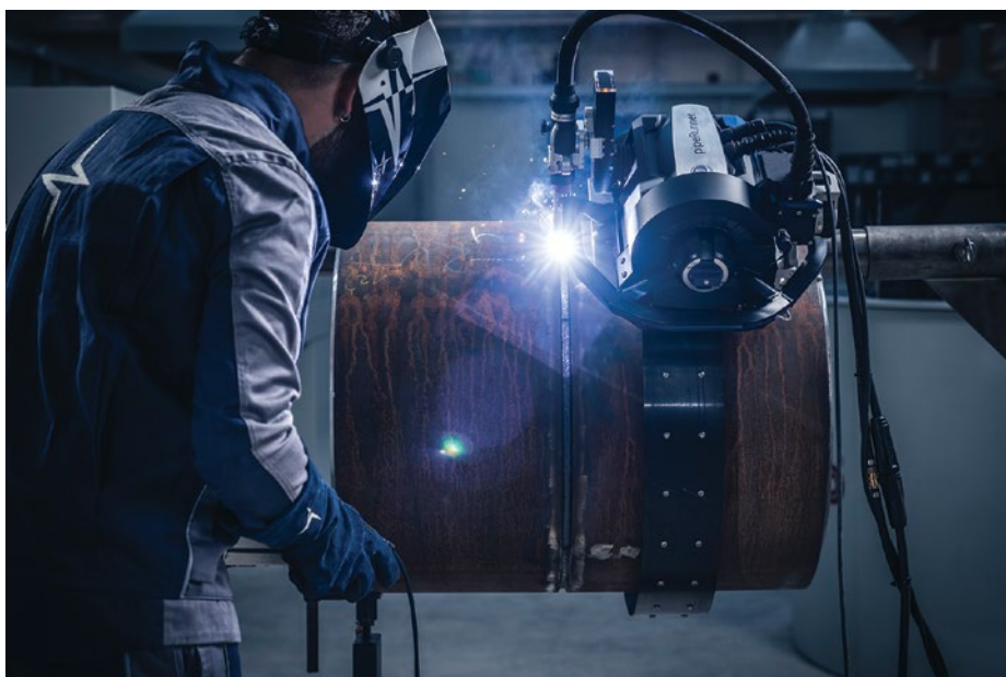
Bohler Welding's new pipeRunner is a state-of-the-art programmable mechanised GMAW/FCAW orbital system designed for girth welding of pipelines and process piping.
