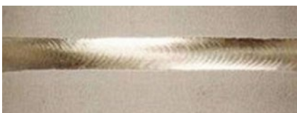
Figure 3b: To ensure no discolouration occurs, the oxygen content needs to be reduced to 20 ppm (0.002%).
