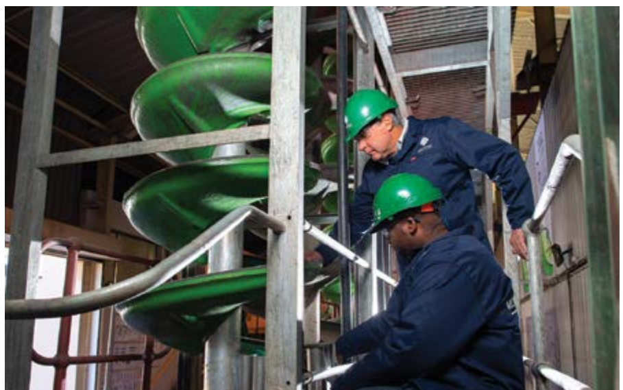
Multotec's versatile spiral test rig in use, upgrading ultra-fine chrome. The full-scale test rig is part of a range of dedicated facilities employed by Multotec's Technology Division to optimise mineral separation and concentration methodologies for customers.
