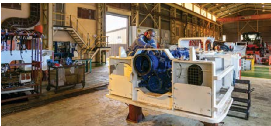
The rebuild of a load-haul-dumper underway at Murray & Roberts Cementation’s Bentley Park rebuild workshops.
