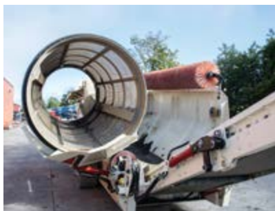
The M518R trommel has a brush cleaner attached to the unit and is especially useful for recycling and light-duty screening applications.
