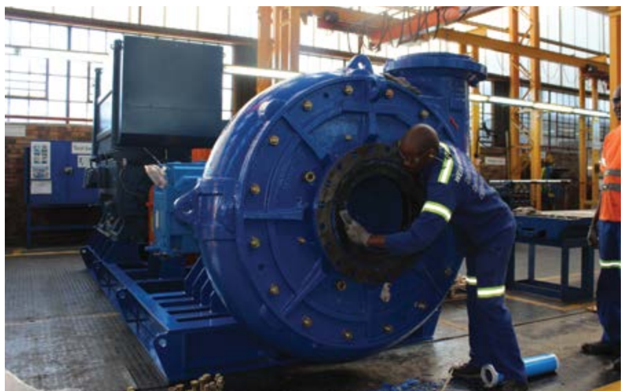
Left: A Warman MC slurry pump under test during developmental stages at one of Weir Minerals' numerous test facilities. Right: A Warman MCU 350 slurry pump being assembled at the Weir Minerals facility in Alrode.
