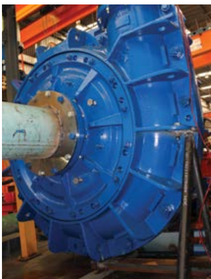
Left: A Warman MC slurry pump under test during developmental stages at one of Weir Minerals' numerous test facilities. Right: A Warman MCU 350 slurry pump being assembled at the Weir Minerals facility in Alrode.
