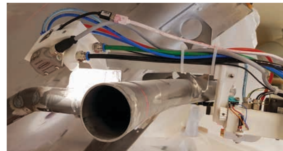
An automated visual (VT) and dye penetrant testing (PT) system with an automated PT nozzle attached to a 3-dimensional head. The manipulator can also be used as a carrier for repair tools as well as end effectors for a J-groove inspection. The system is qualified for nuclear environments.
