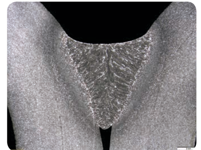
The PCS characteristic features a focused arc that guarantees a deep penetration profile. It is particularly suited to small gaps, fillet welds, and root passes.
