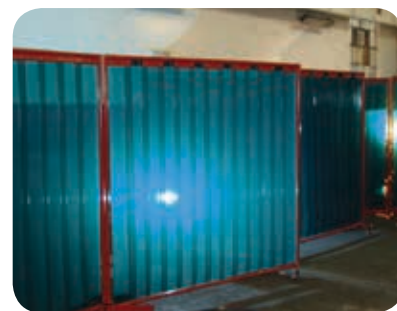
Apex Welding and Safety Screens are used to cordon off welding and grinding bays.
