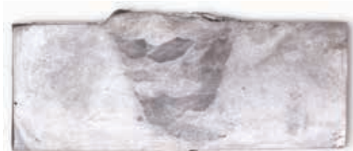
Above and right: Flaw-free macro and bend-test samples of the qualified test piece. “For the first time ever, we have a repeatable welding solution that offers high efficiency while maintaining weld quality,” says Conn Roux of Babcock.
